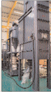
Cyclone, sieve and dust collector
